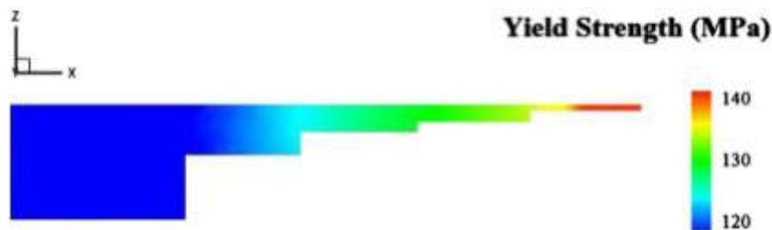
Fig. 12. Distribution of yield strength with 2% SiC in this model.
