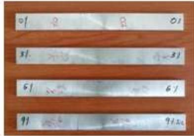
**Figure 2: Tensile test specimens**
