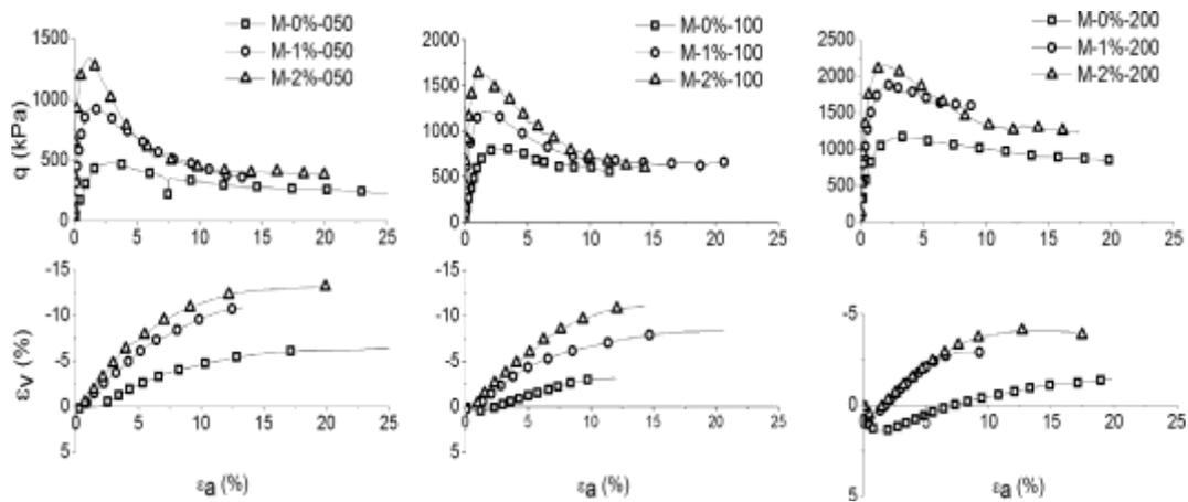
Fig. 6. Comparison of the stress-strain and volumetric responses of the samples with 0%, 1% and 2% cement, under different confining pressures.
