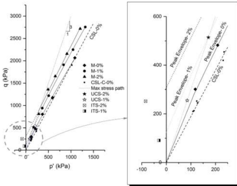
Fig. 10. Peak envelop on  $q$  versus  $p'$  diagram; the inset shows the small stresses region.
