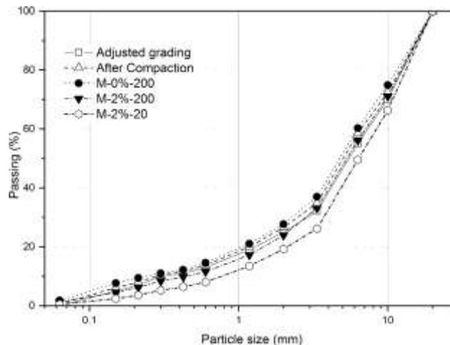
**Fig. 3.** Particle size distributions of the samples: original and after the compaction and monotonic shearing.
