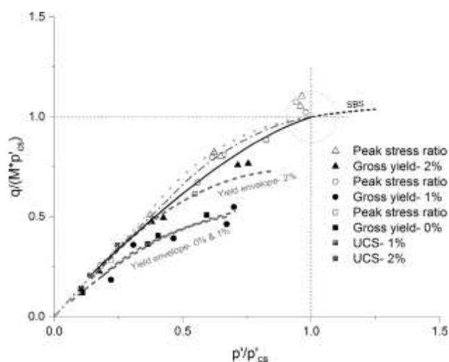
**Fig. 13.** Comparison of the normalized data for the uncemented and cemented soils.
