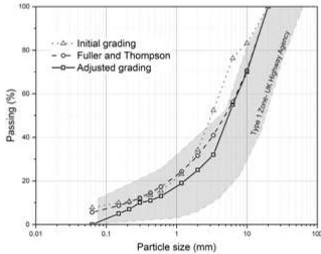
**Fig. 1.** Particle size distributions: Initial grading; Fuller and Thompson(1907)andtheAdjustedgrading. Thegreybanddefinestherangeoftype 1 (UK Highway Agency,2016).
