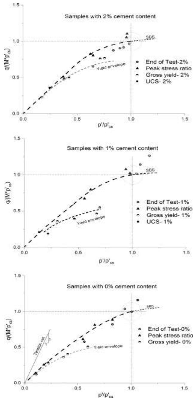
Fig. 12. Normalised yield and strength envelopes: (a) 0%, (b) 1% and (c) 2% cement.
