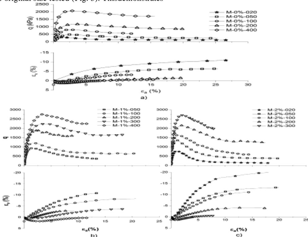
Fig. 4. Stress-strain and volumetric response of the soils tested with: a) 0%, b) 1% and c) 2% cement content.
