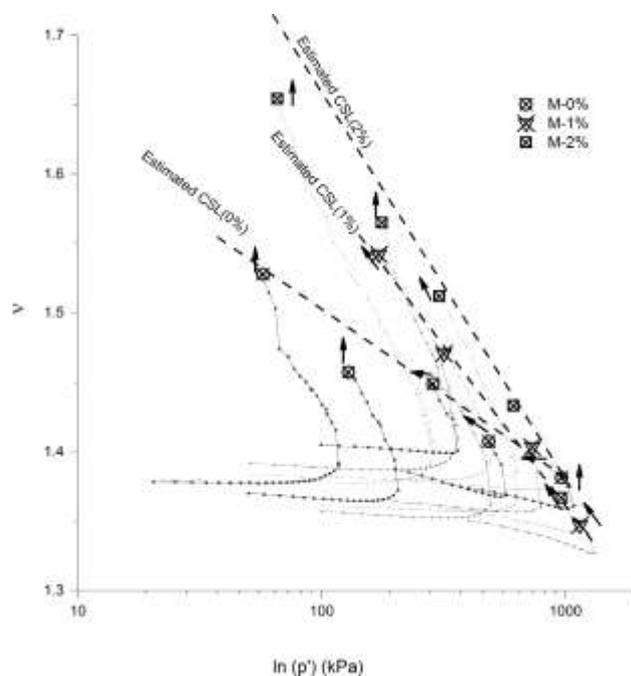
**Fig. 11.** Location of critical state lines for samples with 0%, 1% and 2% cement content on the specific volume,  $m$ , versus the logarithm of the mean effective stress,  $\ln(p^0)$ .
