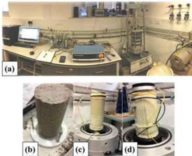
**Fig. 2.** Picture of the equipment and samples: (a) triaxial equipment in the lab; (b) compacted sample in the pedestal and sample with local instrumentation before closing the triaxial chamber.
