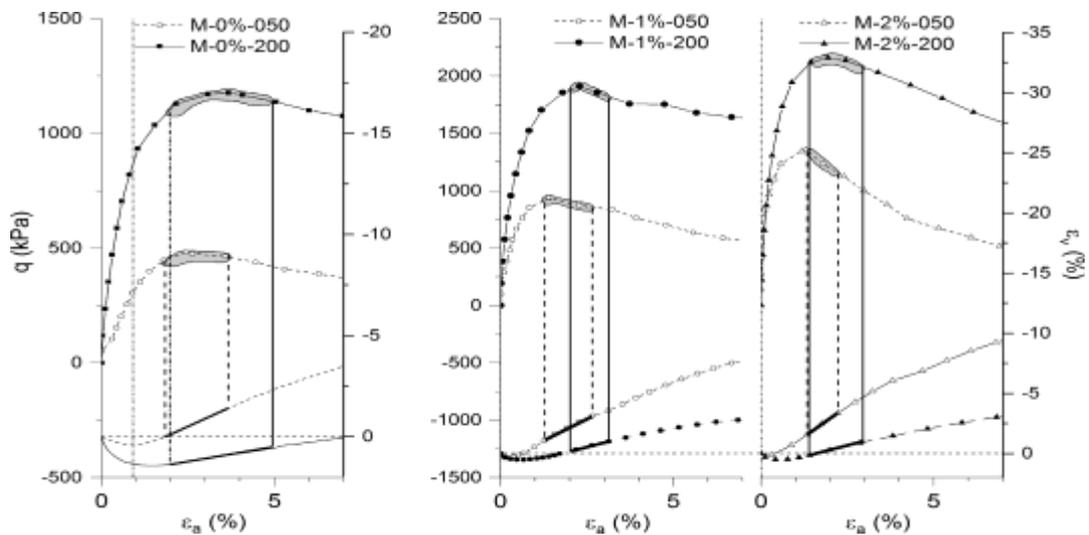
Fig. 7. Relationship between peak stress and maximum rate of dilation for 50 and 200 kPa confining stress: 0% cement on the left; 1% in the middle and 2% on the right.
