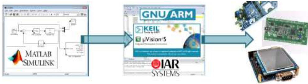
Fig. 5. Simulink® modeling flowchart using the UC3M RCP system. From left to right, Simulink® generates all the required source code for the selected compiler, and automatically loads the resulting firmware into the MCU
