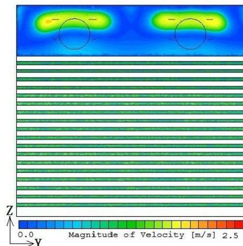
Figure 10 Airflow velocity contours on the Y-Z section of energy-efficient drying kiln
