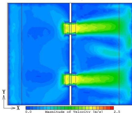
Figure 5 Airflow velocity contours on the X-Y section of conventional drying kiln
