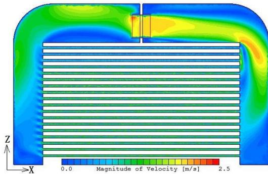
Figure 7 Airflow velocity contours on the X-Z section of conventional drying kiln
