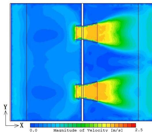
Figure 6 Airflow velocity contours on the X-Y section of energy-efficient drying kiln
