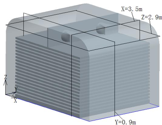
Figure 4 Diagram of each section in drying kiln
