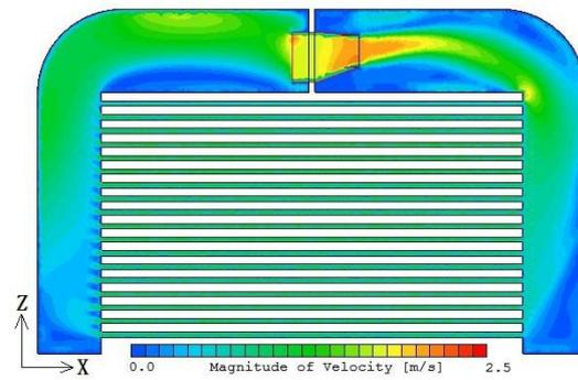
Figure 8 Airflow velocity contours on the X-Z section of energy-efficient drying kiln
