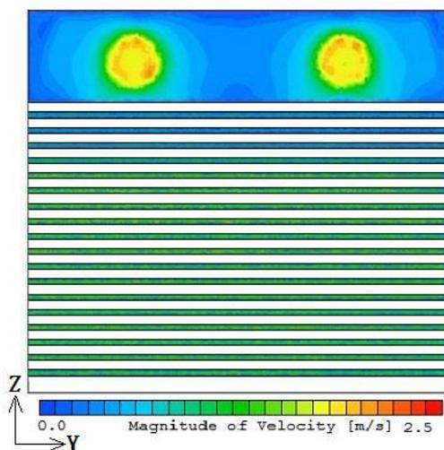
Figure 9 Airflow velocity contours on the Y-Z section of conventional drying kiln
