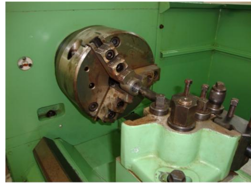
Fig 2: Work piece held in chuck and ready for boring operation
