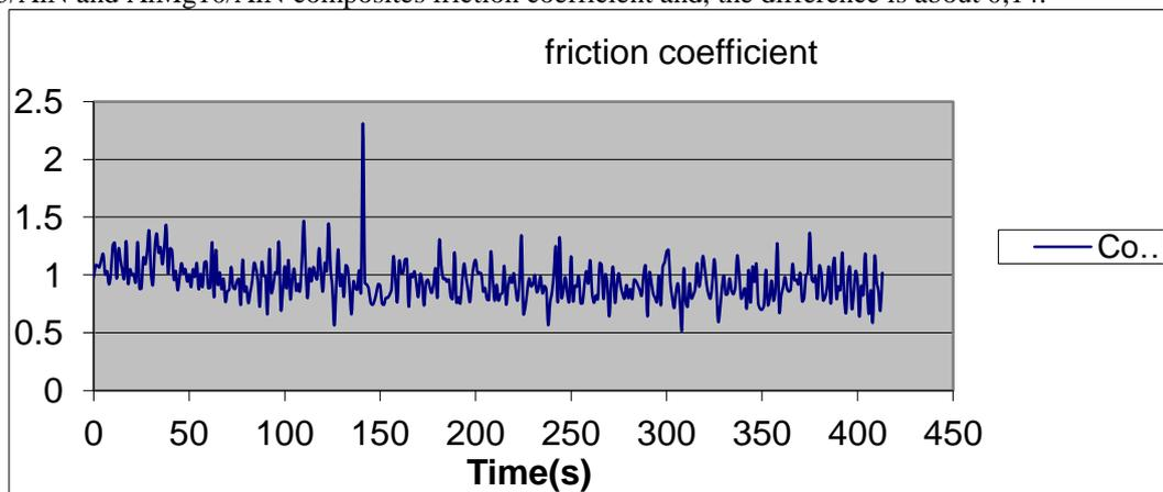
Figure 3. Friction wear coefficient of the AlMg5/AlN composite, value equal with 0,94622
