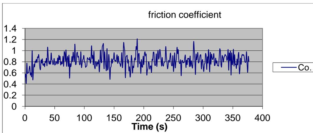
Figure 4. Friction wear coefficient of the AlMg10/AlN composite, value equal with 0,81428
