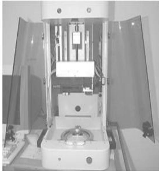
Figure 2. Universal Micro-Tribometer
