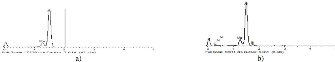
Figure 6.EDS analyses of the composite AlMg10/AlN (microstructures made at laboratories of Politecnico di Torino, Department of Applied Science and Technology)
