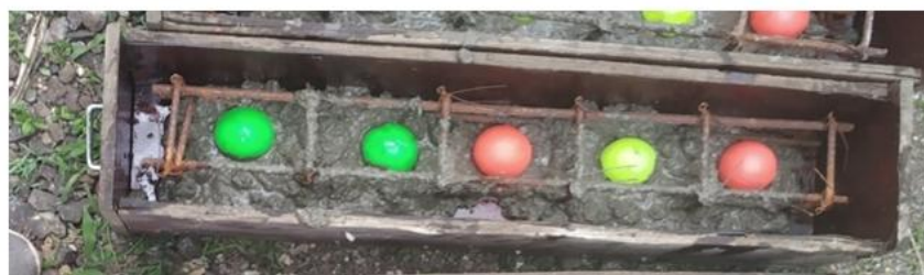
Beam Section with HDPE Ball
