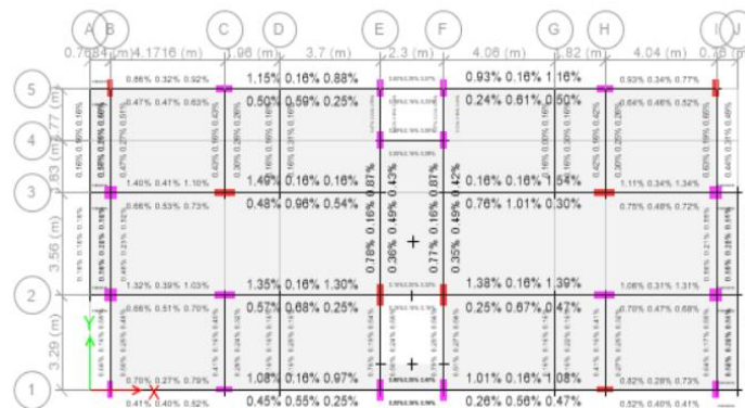
Figure 4. G+9 building members when subjected to seismic loads at MEDIUM SOIL
