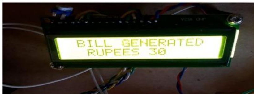
Fig 2: Above snapshot shows the final output of the energy meter ,bill is generated after 4units means 16 counts. For a sample here 30rs generating. Amount is generated as per usage of consumer.
