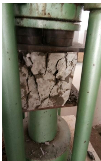
Figure3: Compression test on cube
