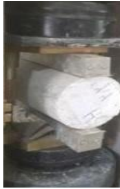
Figure7: Split tensile test on cylinder
