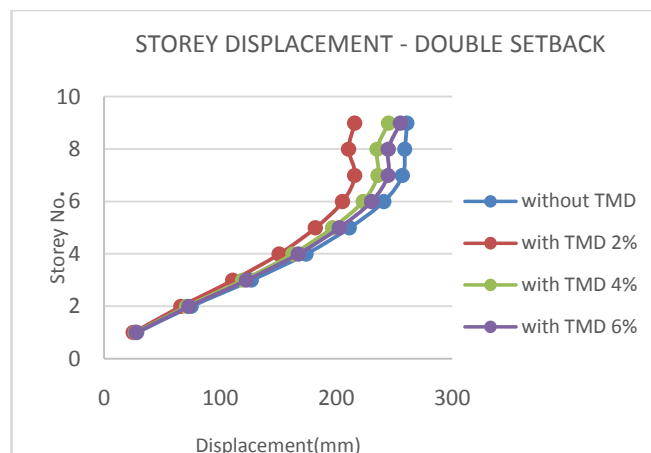
Figure 5: Storey displacement graph of double setback case
