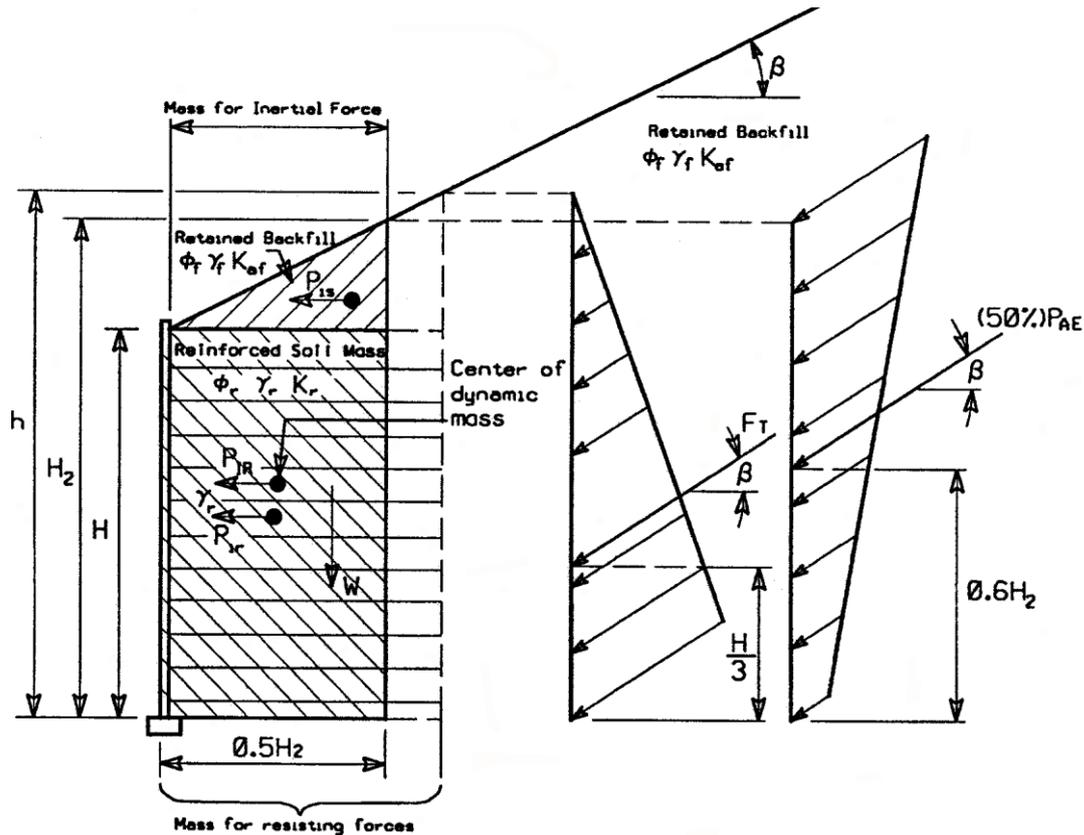
Figure 2.5 Seismic External Stability for Sloping Backfill Condition
