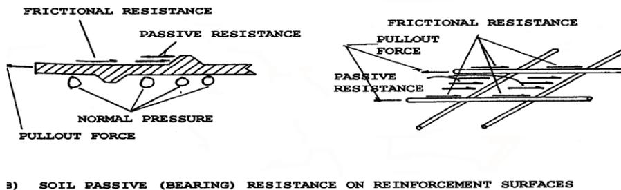
**Figure 2.1** Stress transfer mechanisms for soil reinforcement.(source: FHWA-00-043)
