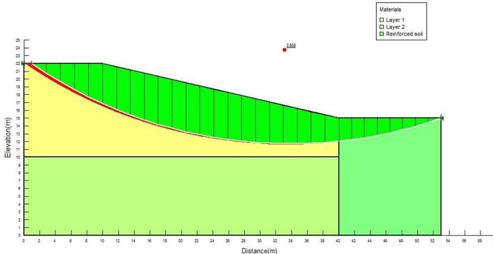
Figure 4.4 Critical Slip circles and Safe Zone
