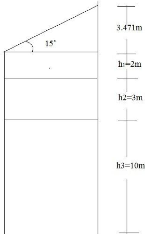
**Figure 4.2 Details of the Backfill Soil**
