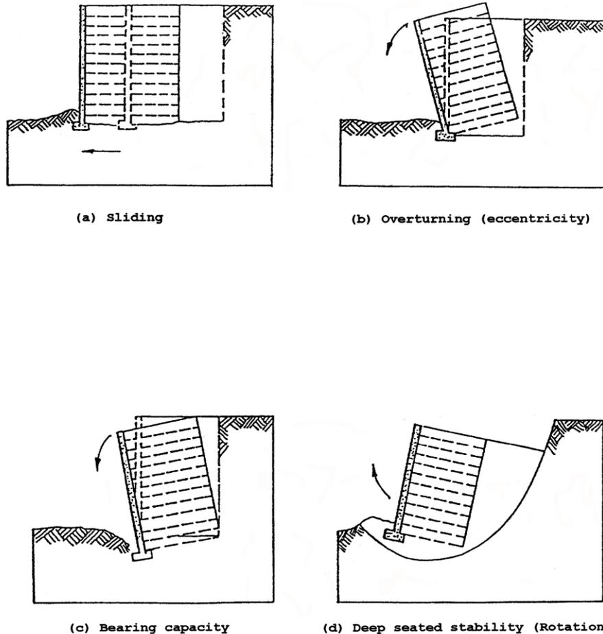
**Figure 1. Potential external failure mechanisms for a MSE wall (source: FHWA FHWA-00-043)**
