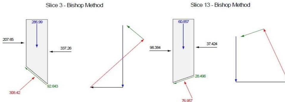
**Figure 3.1: Free body diagram and force polygon for the Bishop's Simplified method** (source: Geoslope 2012)
