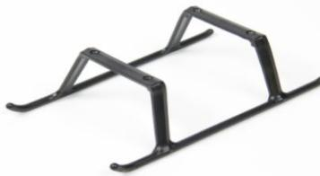
This is a structure meant for safely landing the drone. However, it can be exempted since an experienced user is capable of balancing the motors speed for safe landing in emergencies. There are two major types of landing gear. One is fixed landing gear and the other is retractable landing gear.
