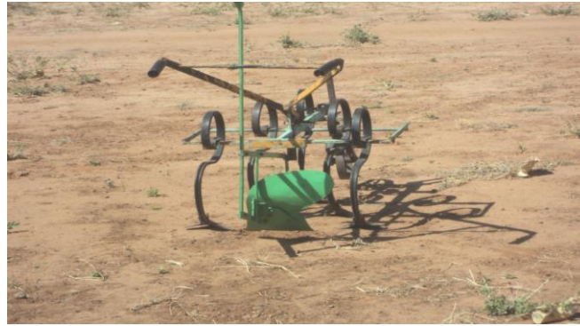
Plate (3) digs (barriers) maker attached to the cultivator
