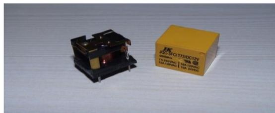
A relay can be defined as a switch. Switches are generally used to close or open the circuit manually. Relay is also a switch that connects or disconnects two circuits. But instead of manual operation a relay is applied with electrical signal, which in turn connects or disconnects another circuit.
