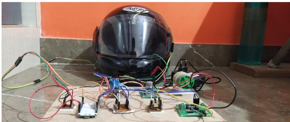
The above snapshot contains all the hardware parts such as Pressure sensor, Alcoholicensor, Tilt sensor , Microcontroller, Dcmotor and Helmet
