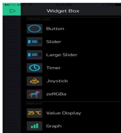
Add a **Button**, then click on it to change its settings. Buttons can toggle outputs on the ESP8266. Set the button’s output to **gp5**, which is tied to an LED on the Thing Dev Board. You may also want to change the action to “Switch.”
