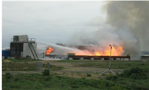
Figure 1: An Example of Open pool fire.
