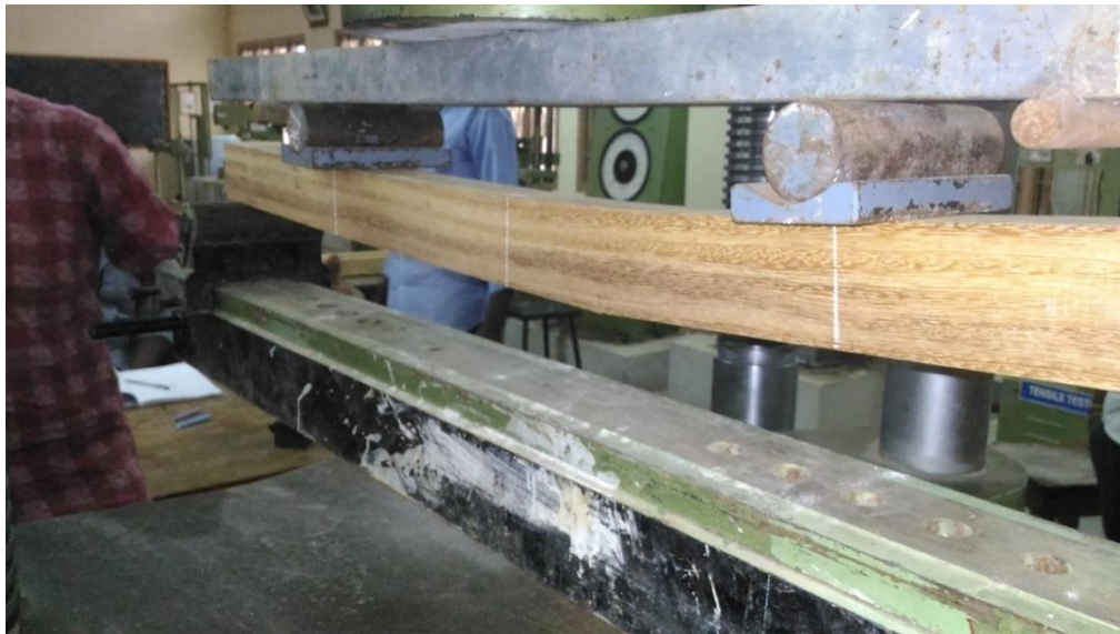
Figure 4 Experimental Setup for flexure test
