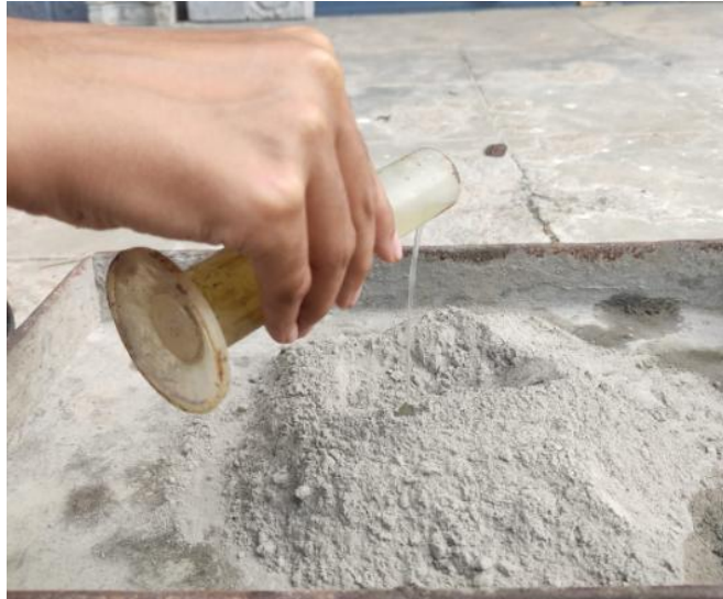
Fig 5.7 Adding of aloe Vera juice to the concrete
