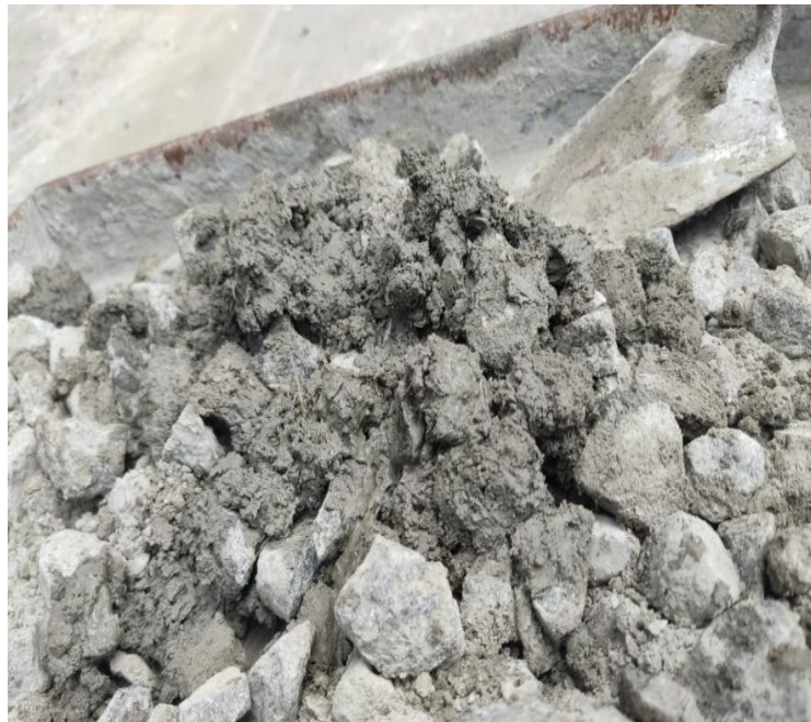
Fig 5.8 Mixing of aloe vera juice with the concrete
