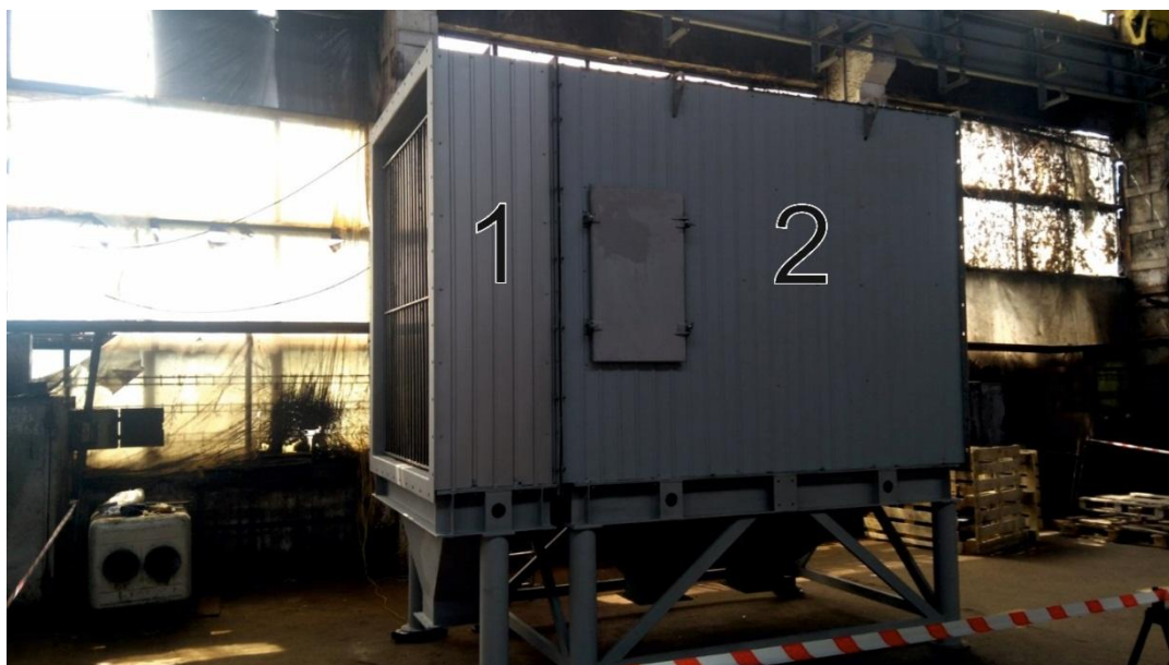
Figure 7: Combined arrangement of gas cleaning unit "MV-2-30"
