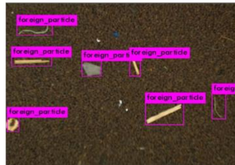
Figure 7. (B) Software output showing the detected foreign matter using YOLO v3
