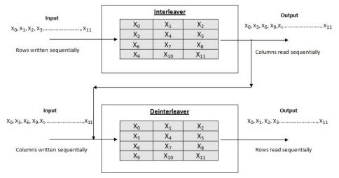
The above interleaver is called as a block interleaver. Here, the input symbols are written sequentially in the rows and the output Symbols are obtained by reading the columns sequentially. Thus, this is in the form of M x N array. Generally, is length of the N codeword.
