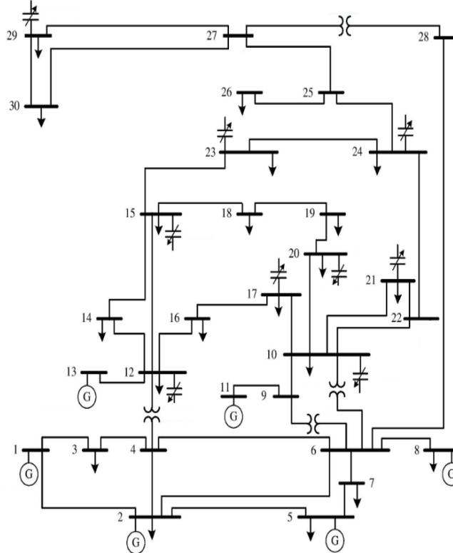
Figure 3. IEEE30-busbar test system [23]
