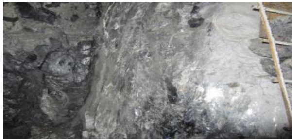
Figure 6: A Karst collapse column in No. 2112 Lane of Tongxin coal mine.
