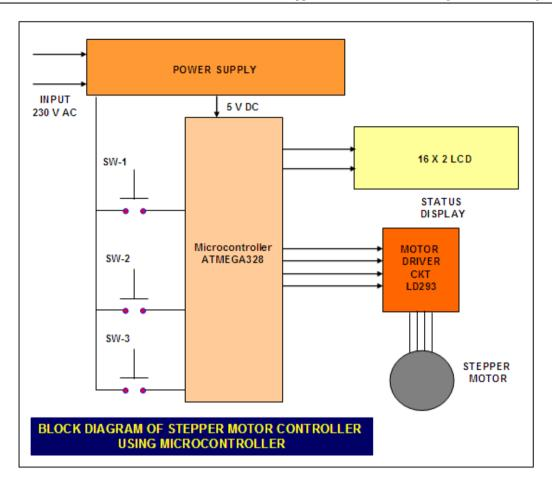
A Stepper motor comes in two types: Unipolar and Bipolar. Unipolar stepper motor generally has five or six wires, in which four wires are one end of four stator coils, and the other end of the four coils is tied together that makes the fifth wire, this is called common wire. Bipolar stepper motor there is just four wires coming out from two sets of coils, meaning there are no common wires.
