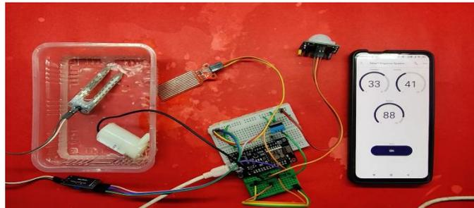
Fig 5: Sensor data reading in Blynk App.
