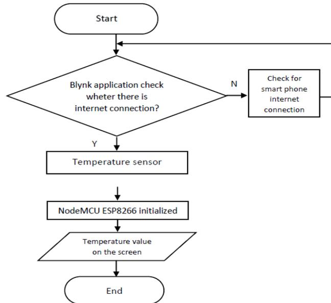
Fig 3: System Flow Design
