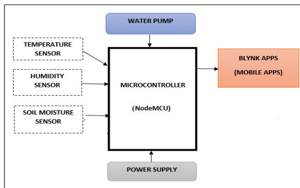
Fig 1: Smart Farming System-Block diagram.
