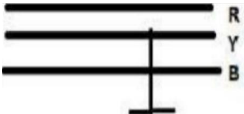
Fig. Line to-Ground Fault
