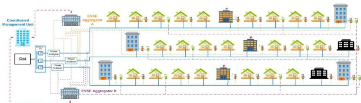
Fig. 2 . Sample power system with coordinated EVSE management
