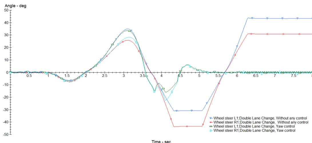
**Fig.10 The front wheel steering angle curve**
