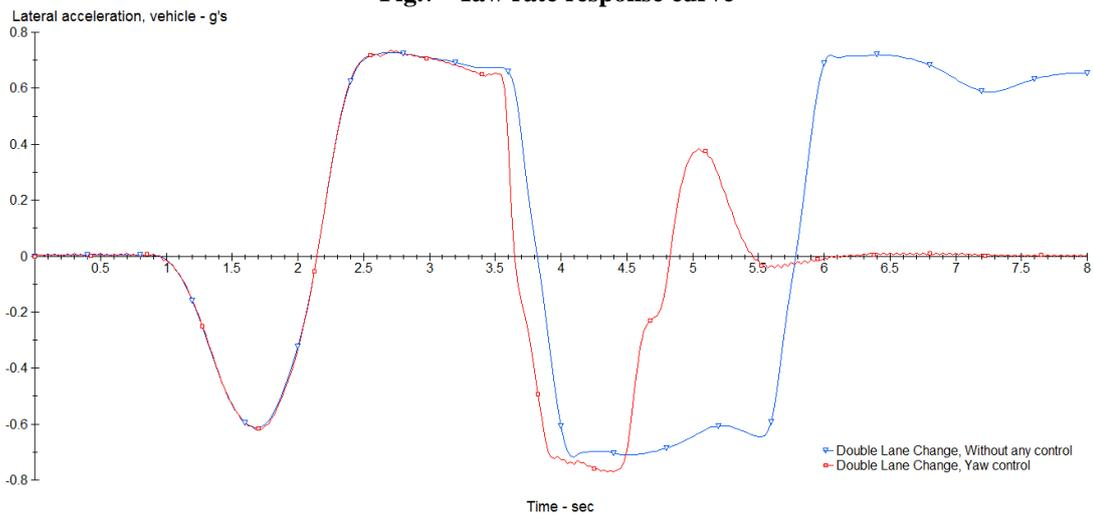
**Fig.8 Lateral acceleration response curve**
