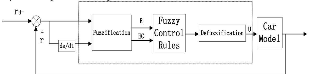
Fig.3 fuzzy controller system block diagram
