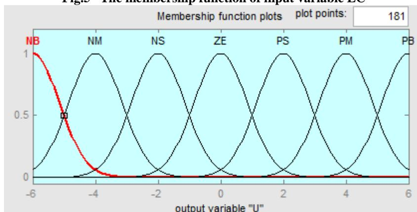
Fig.6 The membership function of output variable U
