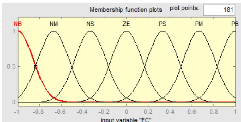
Fig.5 The membership function of input variable EC
