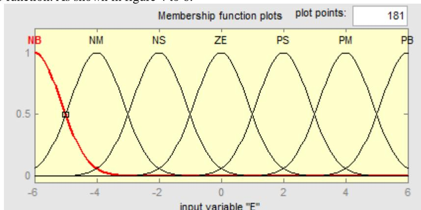
Fig.4 The membership function of input variable E
