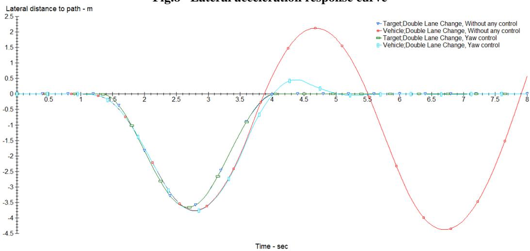
**Fig.9 Target trajectory tracking**
