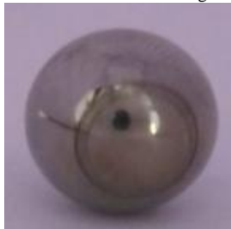
Fig. 5. Ball Wear of SFME+ crude SFO
