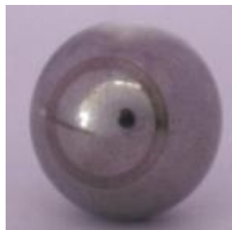
Fig. 6. Ball Wear of 100% 2T Oil
