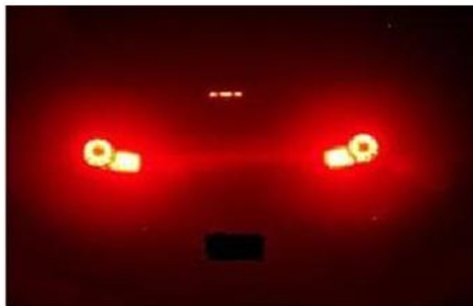
Fig. 1. Tail Lights Cause Camera to Saturate in Places.
