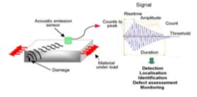
Fig:1 AE sensor working
